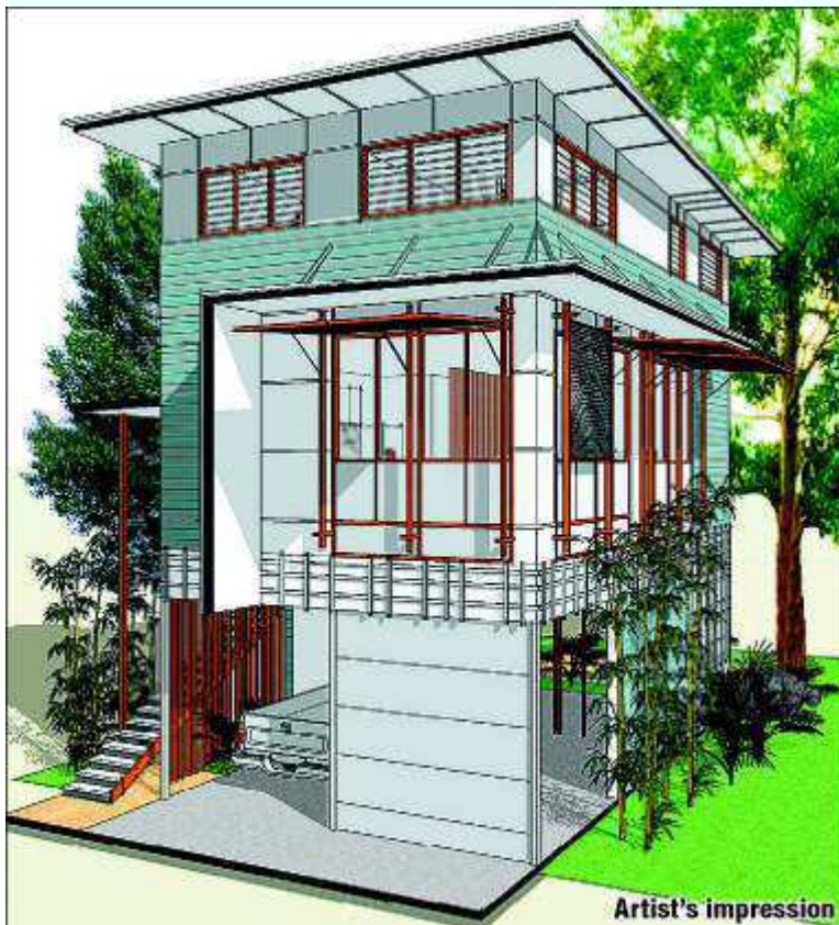
The winning flood resistant design has a high flood-clearance level to the first floor
